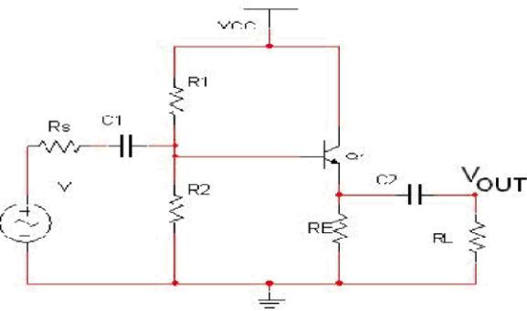
If  $R_1 = 27K$ ,  $R_2 = 5.6K$ ,  $RL = RE = 220$ ,  $RS = 0$ , Find the maximum undistorted peak-to-peak output voltage.
