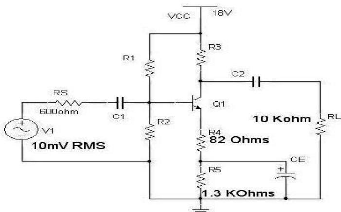
b) Analyse what the output voltage should be if the DC power supply given to a CE amplifier is shorted to ground.
